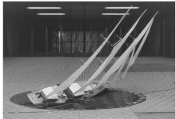
Figure 2. A model sailing yacht in a large environmental tunnel
