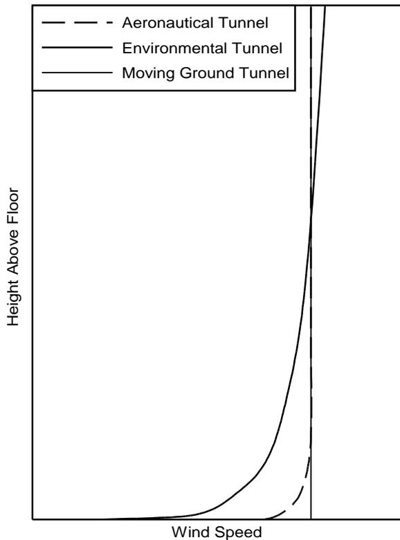
Figure 4. Typical velocity gradients found above the floors of wind tunnels
