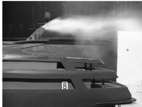
Figure 9. Exhaust plume trajectory interfering with the aft end of the sun deck
