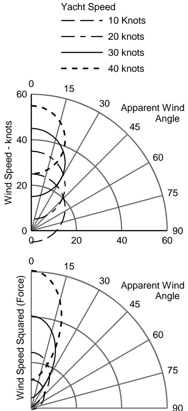
Figure 11. The apparent wind speed and direction on board a yacht travelling in 15 knots true wind, with true wind angles ranging from ahead to astern.
