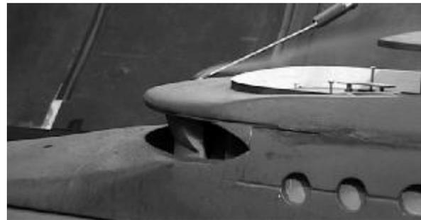
Figure 13. A screen fitted to deflect wind upwards and improve the wind comfort in an area of exposed seating
