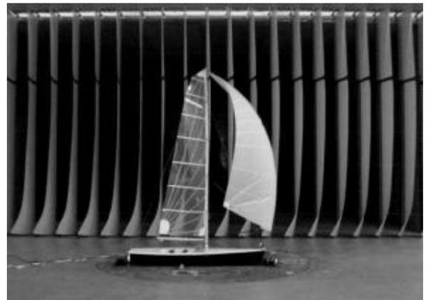
Figure 5. A racing yacht model in the Auckland University twisted flow tunnel
