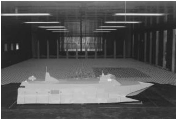
Figure 15. A catamaran ferry on a 6 component balance in the tunnel floor
