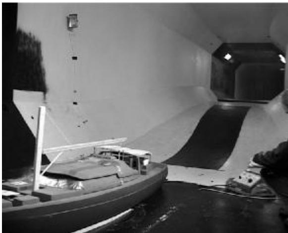
Figure 1. View from the low to the high speed section of one of Southampton University's aeronautical tunnels
