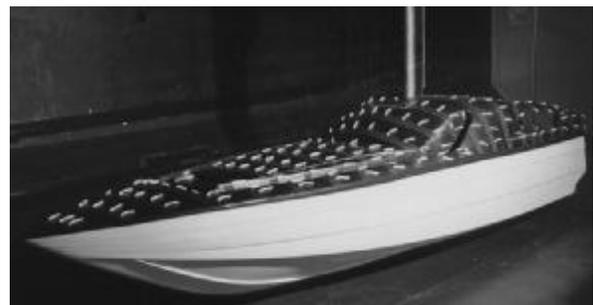
Figure 6. Wool tufts to visualise surface flow pattern
