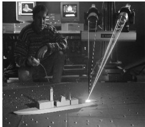
Figure 8. Laser doppler anemometry on a flight deck in the Bristol University tunnel
