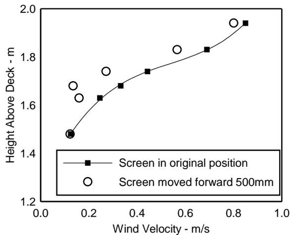
Figure 12. Variation of local wind speed with height at the fly bridge helm position
