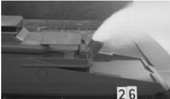
Figure 10. Study of alternative gas turbine exhaust arrangements
