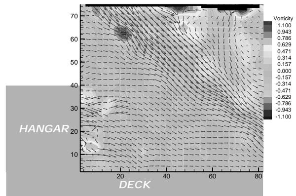
Figure 14. PIV measurement on the centreline plane of a naval vessel during helicopter approach
