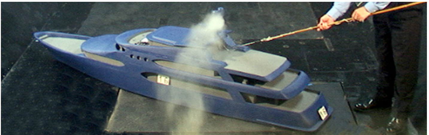
Exhaust plume trajectory wind tunnel tests - Laurent Giles Naval Architects Ltd
