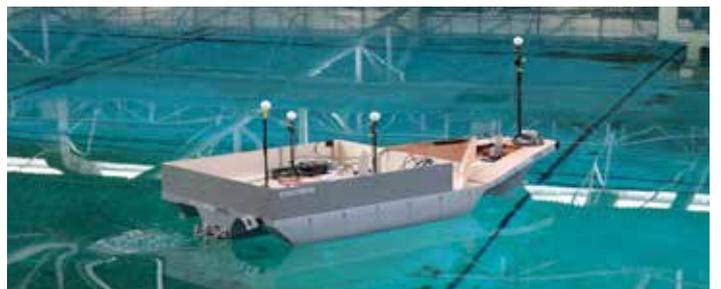
Manoeuvring trials on a 24m SWATH Trimaran designed by AUSTAL Pty
