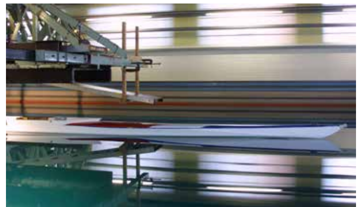
Towing tank testing of a rowing shell
