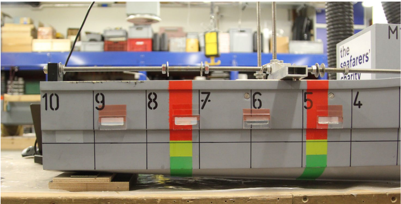
Figure 5 Starboard view of M1204, decked vessel variant with non-return flaps fitted
