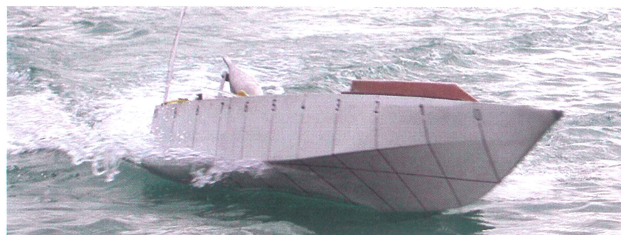
Fig 3. Manoeuvring tests on a patrol craft with twin waterjets.
