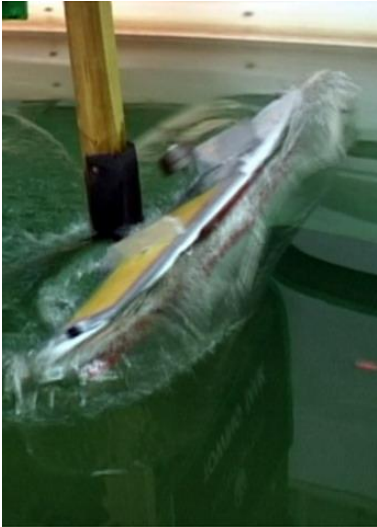
Figure 13. Marchioness, decked, 6 knots, 1.6 seconds after impact
