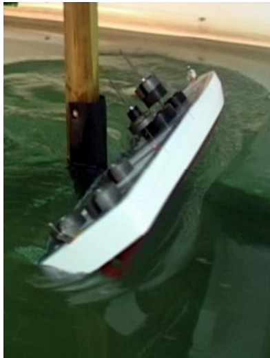
Figure 16. Wider vessel, high VCG, 4 knots, 4.0 seconds after impact
