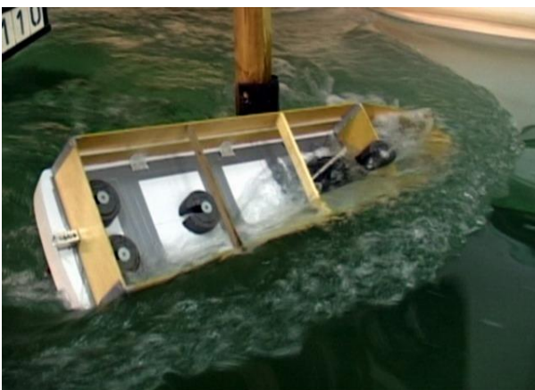
Figure 18. Wider vessel, high VCG, with superstructure, 8 knots, 9.6 seconds after impact
