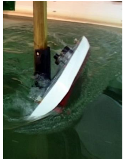
Figure 17. Wider vessel, low VCG, 6.5 knots, 4.0 seconds after impact
