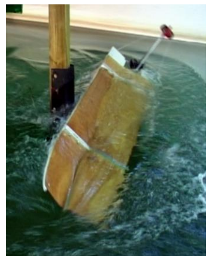
Figure 19. Catamaran, 6 knots, 3.6 seconds after impact
