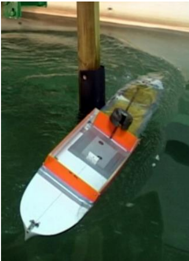
Figure 15. Marchioness, with aft superstructure, 4.5 knots, 6.4 seconds after impact
