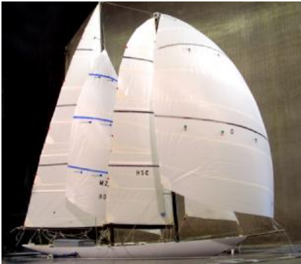
Figure 5 Typical multi-sail wind tunnel set up. (Courtesy Hoek Design).
